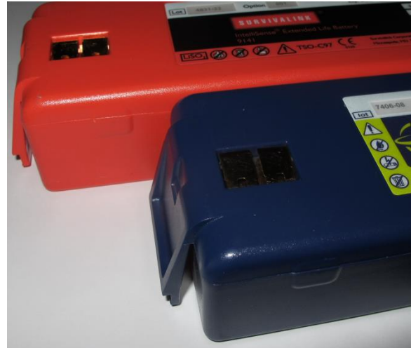
Figure 2. Snap fit design feature of the AED lithium batteries in two colors: warm red C and dark blue
